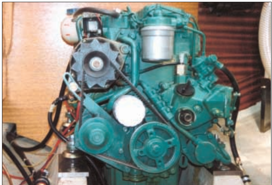
Example of RAB-installation on a 3-cylinder diesel engine power pack.
