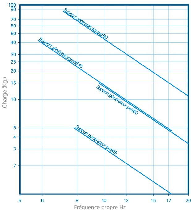
COURBE DE CHARGE-FLÈCHE AMC MECANOCAUCHO®
